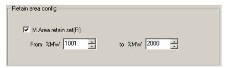
• In addition to the above two, symbolic variables (named variables) occupying 512KB of data memory (local and global) can be individually configured for memory retention during variable declaration phase.
