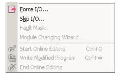
Any part of the PLC program can be edited online when CPU is running & the new program can be downloaded to the CPU without having to stop the CPU.
